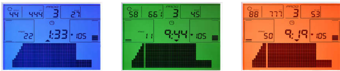
Fig.4: Multicolor backlight function for a visual indication of workout target.
