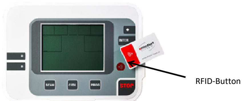
Fig. 5: RFID-button for RFID identification, in case the medium cannot be read via the slot
