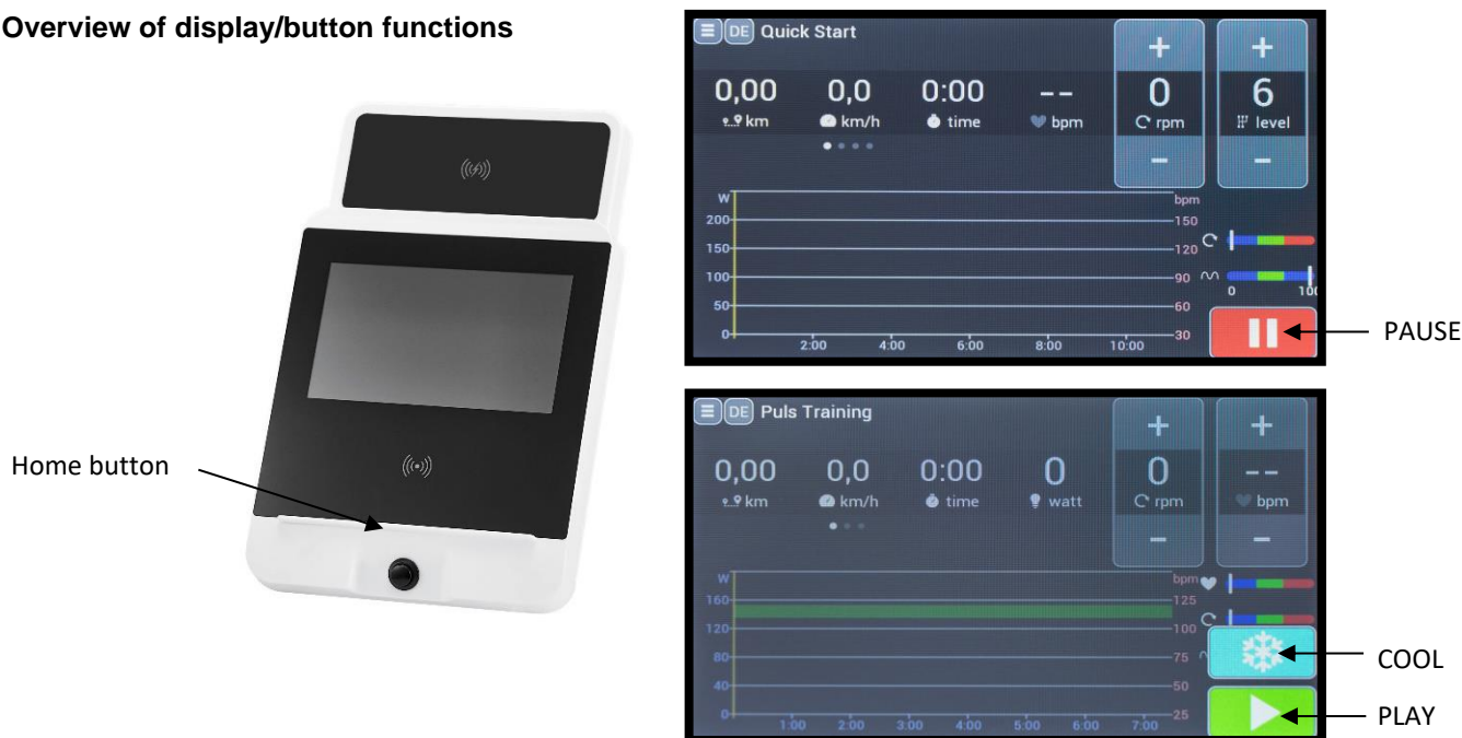
Fig. 9: Monitor view, to explain the button functions, actual view may vary in colour, button assignment is the same.
