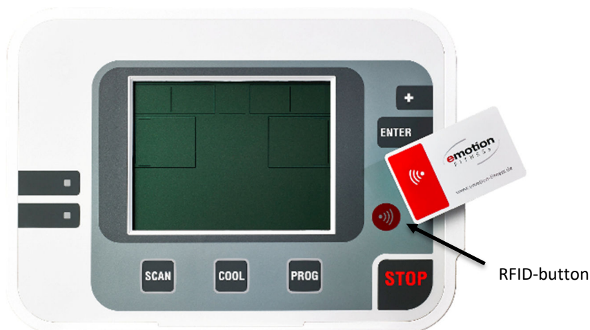
Fig. 5: RFID-button for RFID identification, in case the medium cannot be read via the slot
